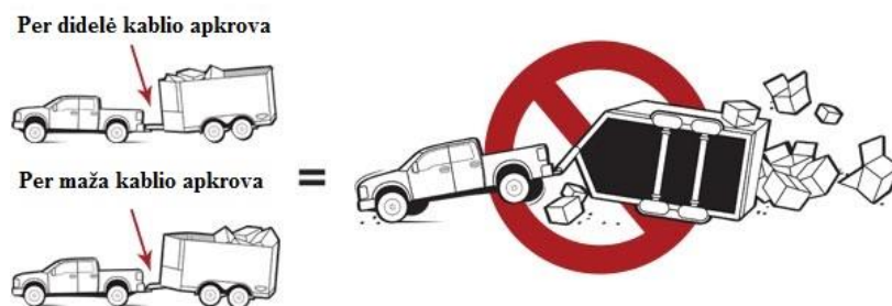
3 pav. Sukabinimo taške susidarančios masės įtaka saugiam eismui (Šaltinis: https://www.weigh-safe.com ) Fig. 3. Influence of the mass produced at the coupling point on safe traffic (Source: https://www.weigh-safe.com )
